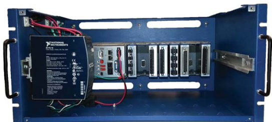
FIG. 1. cRIO system inside National Instruments chassis.
